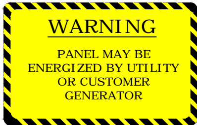
TAG 1: Install on Meter Box
